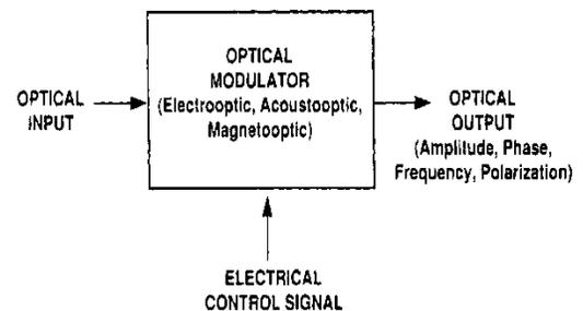
Figure 1. Solid-state optical modulator, in which the optical signal is modulated by applying an electrical control signal.
