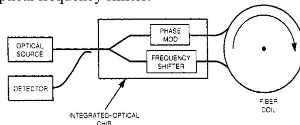
Figure 6. Fiber-gyroscope multifunction integrated optical chip.
