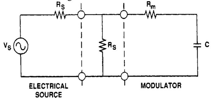
Figure 3. Lumped-element equivalent-circuit model of an electrooptic modulator system. The capacitor voltage corresponds to the modulator electrode voltage.
