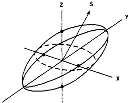
Figure 2. As light propagates through a crystal, the two allowed states of linear polarization associated with a propagation direction *s* are parallel to the axes of the ellipse formed by the intersection of an ellipsoid and a plane perpendicular to *s*.
