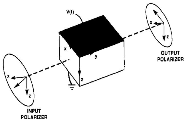
Figure 4. Bulk electrooptic intensity modulator consisting of an input polarizer oriented  $45^\circ$  with respect to the modulator axes, a polarization-dependent electrooptic phase modulator, and an output polarizer oriented  $90^\circ$  with respect to the input polarizer.
