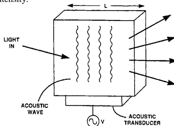
Figure 5. Bulk acousto-optic modulator operating in the Raman-Nath regime, in which the acoustic wave perturbs the optical beam resulting in multiple diffracted beams.
