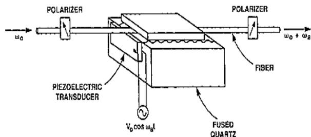
Figure 8. Fiber optic frequency shifter in which an acoustic wave from a transducer perturbs the two guided modes of a high-birefringence fiber, causing mode coupling.
